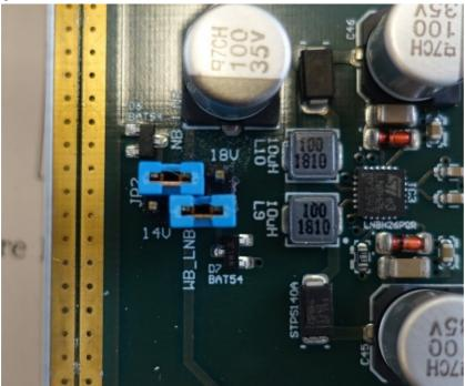
This sets the narrowband LNB channel (upper jumper, left position) to vertical polarization (14V) and the broadband LNB channel (lower jumper, right position) to horizontal polarization (18V). This should be sufficient for most users in Europe. Users in South America or Southeast Asia can exchange this configuration.
