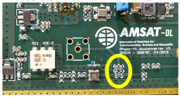
This can be easily fixed by removing all three 50 Ohm resistors in the yellow circle area. This can be done with a soldering iron and a large amount of solder, so that all parts can be heated at the same time and pushed to the side with the soldering iron. It is then necessary to reconnect the SAW filter output to the conductive path leading to the F connector using a short piece of wire or a large solder blob.
