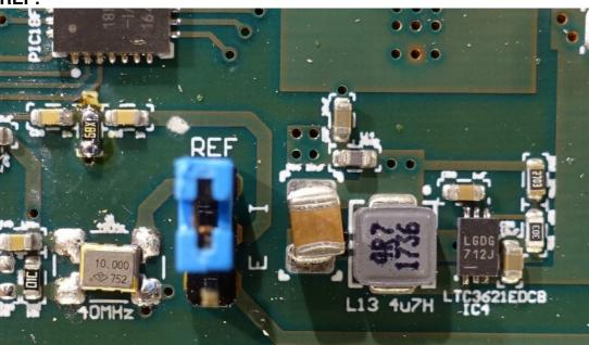
The REF jumper in the upper position connects the internal TXCO with the LO. This should be fine for most users. Users with extremely stable references (Rubidium or GPSDO) can use the lower position and add an SMA jack on the right side of the PCB.
