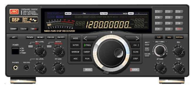
If you press FUNC then WIDE, you can assign a different bandwidth value to the WIDE button. Same goes for FUNC + INTER and FUNC + NARROW. (There's nothing to stop you assigning a wider bandwidth to the NARROW button, as compared to the value assigned to the WIDE button. For example, WIDE may be set to 2.5 kHz and NARROW might be set to 5 kHz!).
