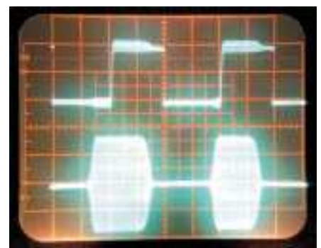
Figure 3—CW keying waveform for the TS-2000 showing the first two dits using external keying. Equivalent keying speed is 60 WPM. The upper trace is the actual key closure; the lower trace is the RF envelope. The transceiver was being operated at 100 W output at 14.02 MHz.
